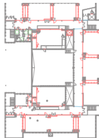
Third Floor Demolition Plan
